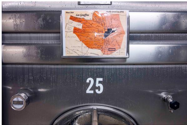
Each part is sent to a specific stainless steel tank. It will have, right from the beginning, its own ID. They will remain there for 12 hours, allowing a natural clarification to take place. The heavier particles in the juice will fall at the bottom of the tank and the clear juice will remain on top. The juice will then be pumped and transferred to another tank to begin the alcoholic fermentation.
